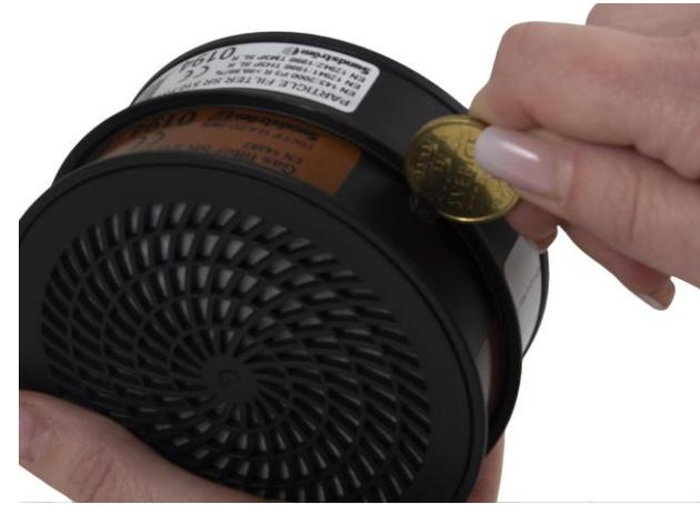
**2.3** Place a coin between the lower lip of the particle filter and the small tab molded into the side of the gas filter. Push firmly and twist the coin until the filters separate.
