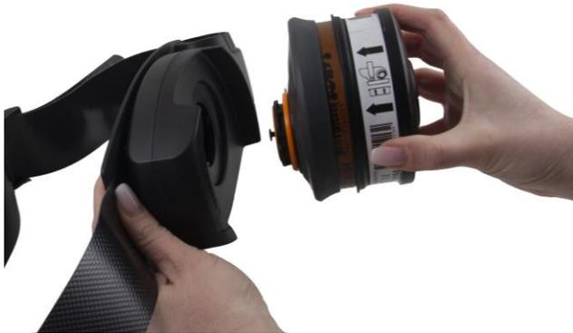
Inspect all parts and replace with new parts as necessary. Critical areas are the membranes and the connections/attachments which must have clean and undamaged contact surfaces.
